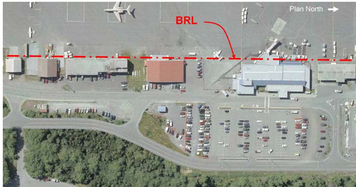
Fig. 5. 2009 Aerial Photo of Sitka Rocky Gutierrez Airport, Terminal Area. Note building restriction line (BRL) demarks westerly limit of building construction.
